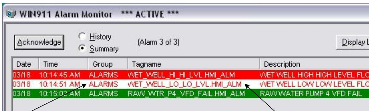
STEP 1: Write down the tag name that you wish to bypass and the group that that alarm is in. To find the tag name open the WIN-911 Alarm Monitor and find the tagname under the tagname column.
